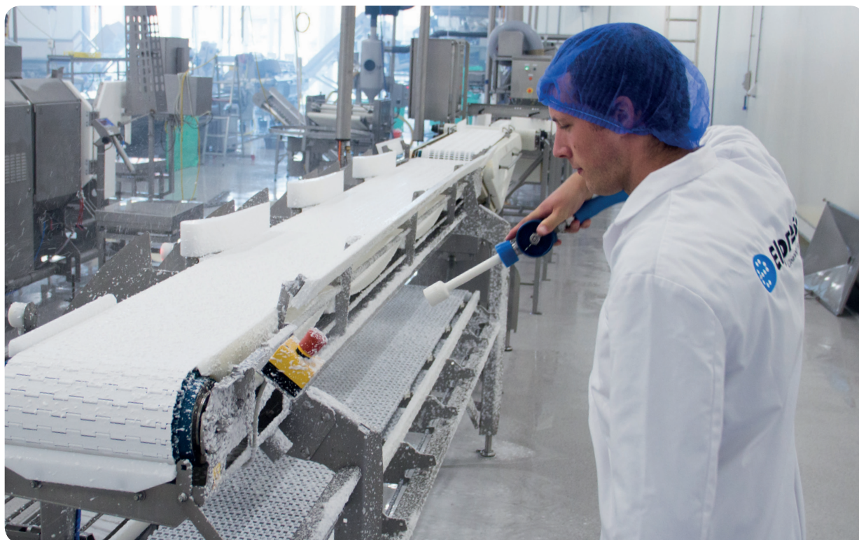
The CF-Q 6E enables up to 6 users to foam at the same time.
